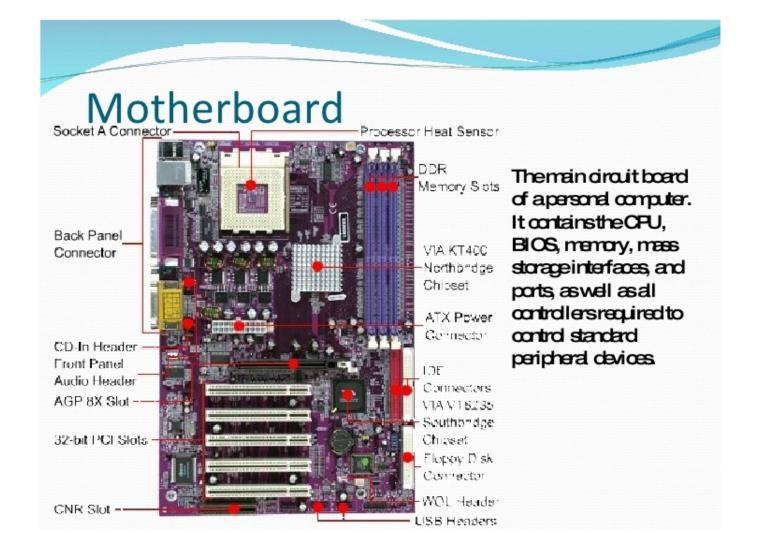
Is The Motherboard The Main Circuit Board Of The Computer
